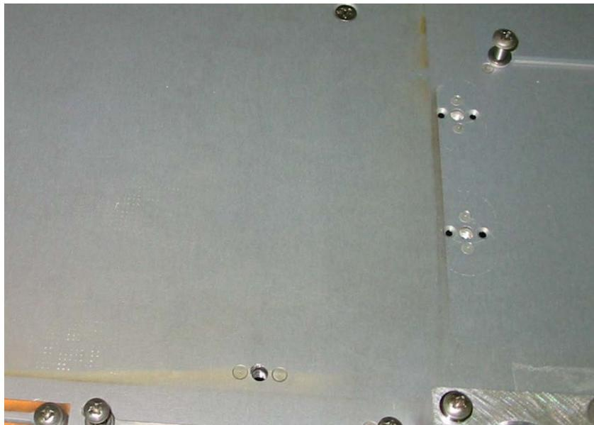
Figure 4. Deposition on MISSE baseplate from composite sub-experiment.
