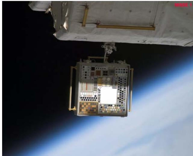
**Figure 2. Shadowing of MISSE-1 by the airlock**
