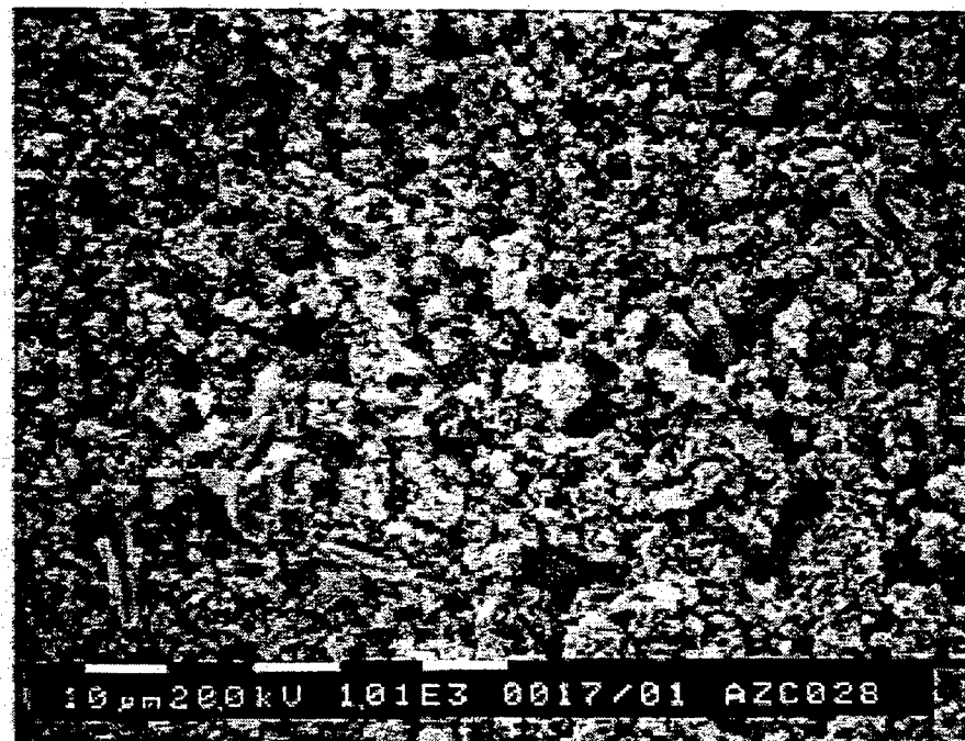
Figure H-12. 500x & 1000x SEM Image of AZC028, 500 Angstroms Tefzel on Z93 White Ceramic Paint, Flight Exposed Sample
